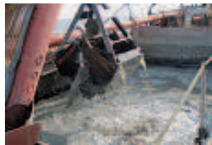
Sediment slurry in a dredger, ready for dispersion at the test site
